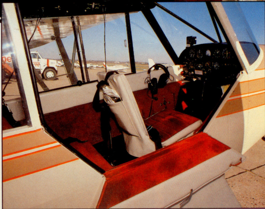
The Cub's panel arrangement is logical and relatively uncrowded, a tribute to the technicians at Ransome Avionics. Ransome's Apollo II Loran is the preferred method of navigation: Course information can be channeled to HSI.
